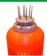
The VP-LED is a spar buoy lantern developed for integration on polyethylene plastic spar buoys and it will withstand moderate ice conditions. The lantern housing is made of epoxy painted marine grade aluminium alloy, and the complete unit has a weight of only 4 kg's.
